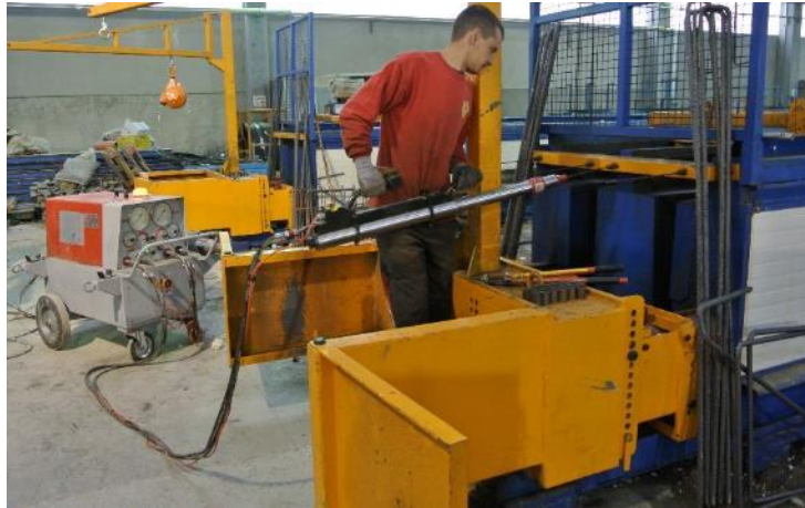
Hydraulic pumps for stressing and relaxation of strand; barrels and wedges for strand.
